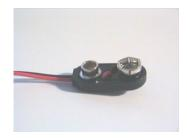
Solder the 9v battery cable to the +9v and GND hole.
