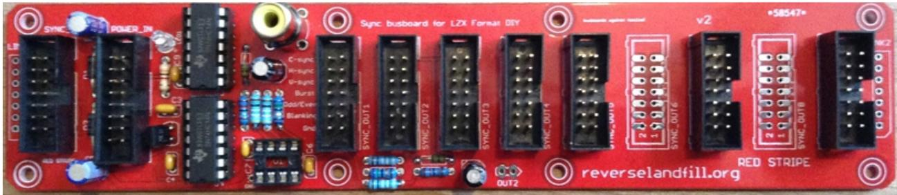
This buffered sync busboard is designed for connecting several Cadet / DIY modules that use the 14 pin sync bus. You need a Cadet Sync generator or Visual Cortex as sync source.
