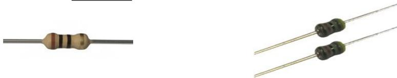
The one **10R** resistor has the color code: 'brown-black-black'. It is used at the power input as a fuse. Bend the legs of the resistor 90 degrees and place the **10R** resistor at the **R1** location on the PCB. Solder the resistor and cut off the legs with a sidecutter.
