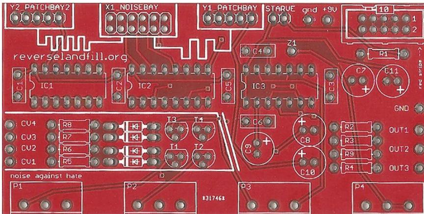
The Noise! Synthesizer is a CMOS IC based instrument. The synth has 4 squarewave oscillators that modulate each other and go through a clock divider. After that, the separate divider outputs are mixed and shaped together. Then the signal is routed through a pseudo ringmod.
