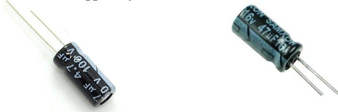
These parts have a **polarity**. The long leg is the PLUS, The short leg is MINUS. There is also a MINUS symbol printed on the side. The value of these components is printed on the side as well.
