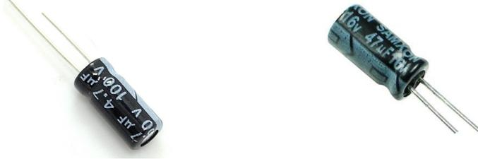
These parts have a **polarity**. The long leg is the PLUS, The short leg is MINUS.
