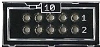
Place the 10 pin eurorack connector. The open side goes up, with "10" marking on the PCB .
