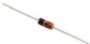
There are four zener diodes. These make sure that the CV input voltage cannot be higher than 9.1 volt.
