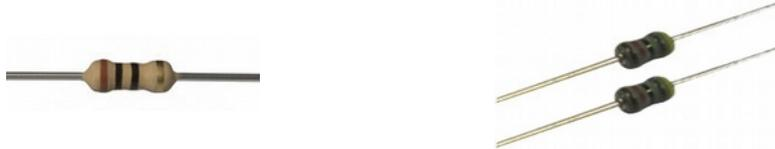
The one **10R** resistor has the color code: 'brown-black-black'. It is used at the power input as a fuse. Bend the legs of the resistor 90 degrees and place the **10R** resistor at the **R1** location on the PCB. Solder the resistor and cut off the legs with a sidecutter.
