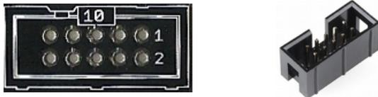
Take the 10pin shrouded header and solder first one pin. Check is the header is flat to the pcb. Reheat if necessary. Then solder all pins.
