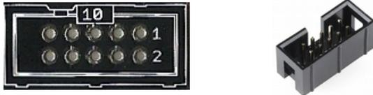
Take the 10pin shrouded header and solder first one pin. Check is the header is flat to the pcb.
