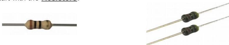
The one **10R** resistor has the color code: 'brown-black-black-gold-brown'. It is used at the power input as a fuse. Bend the legs of the resistor 90 degrees and place the **10R** resistor at the **R1** location on the PCB. Solder the resistor and cut off the legs with a sidecutter.
