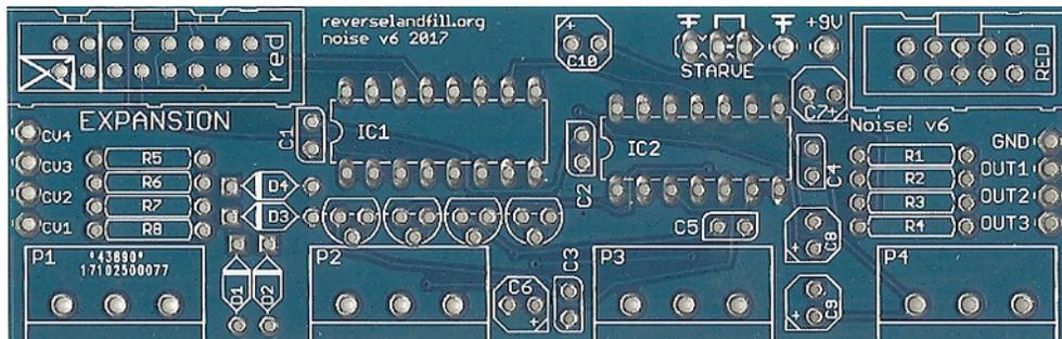
The Noise! Synthesizer is a CMOS IC based instrument. The synth has 4 squarewave oscillators that modulate each other and go through a clock divider. After that, the separate divider outputs are mixed and shaped together.
