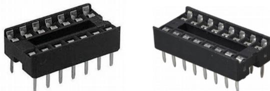
These IC-sockets are to make the placement (and possible removal) of the IC's easier. Take out the *two* IC-sockets. Attention! These sockets have a direction. See the semi-circle gap?
