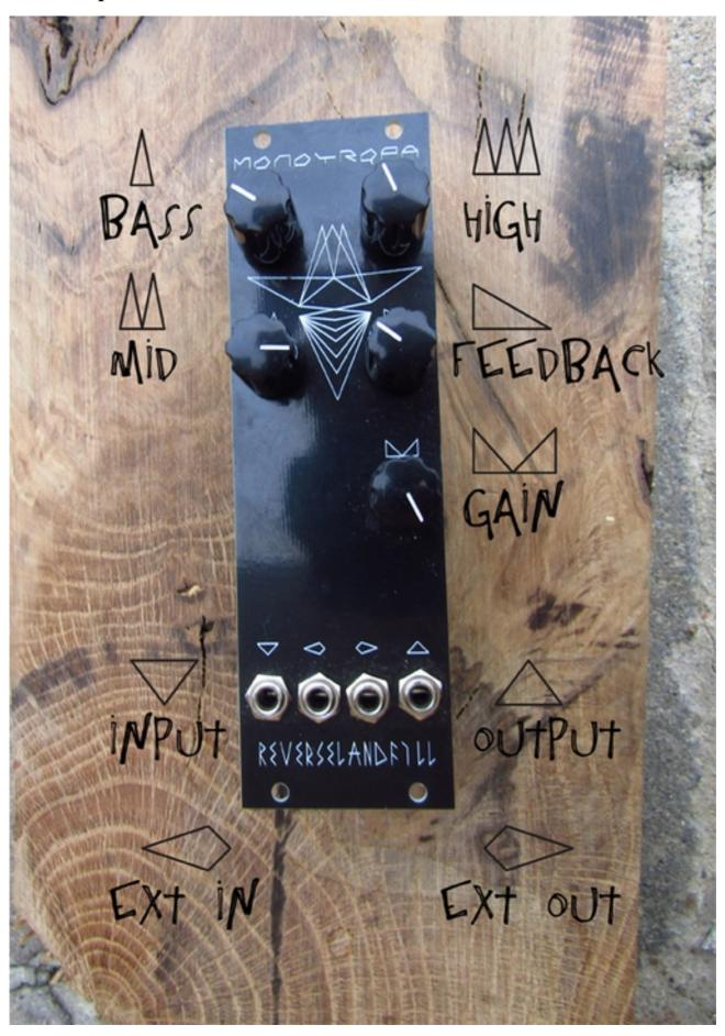
Monotropa is a 3 channel equalizer with a feedback path and 10x gain.
